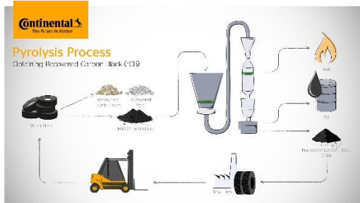
Continental PP Pyrolysis process EN
